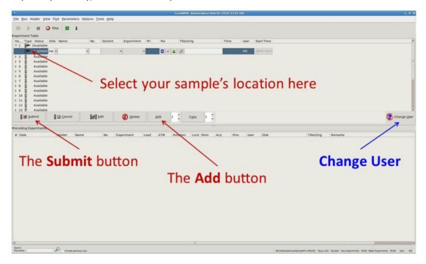
If you want to run multiple experiments on the same sample, make sure you have that position selected and click the Add button. Fill out the necessary information. Once you have entered all of the samples you want run, hold down the Shift button and select all of the experiments you want run. Then click the Submit button. This will start the run.
